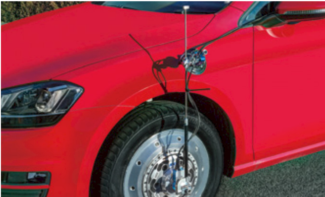
The WFS Wheel Force Sensor measures the six-component forces of a vehicle in dynamic conditions.
